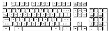
Figure 5-1 A 101-key enhanced keyboard layout
